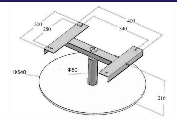
From floor to top of plate: 216mm Swivel Column: 50mm Base Diameter: 540mm Mounting holes pitch: 250x340mm Chassis size: 300x400mm
